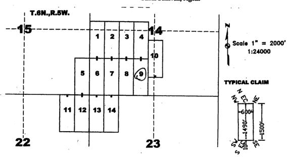
The above map depicts the LM \_\_\_\_\_\_ lode mining claim, which is located in Section(s) \_\_\_\_\_\_, Township 6 North, Range 5 West, Gila and Salt River Baseline and Meridian, Maricopa County, Arizona. The claim corners, end centers, and location monuments are marked by 2 inch by 2 inch by 5 foot wooden posts with aluminum tags. The bearings and distances between claims are as depicted on the map.
