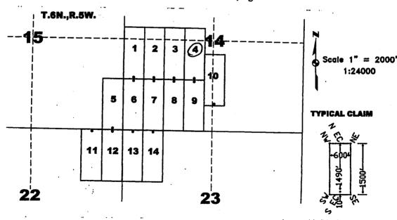
The above map depicts the LM lode mining claim, which is located in Section(s) North, Range 5 West, Gila and Salt River Baseline and Meridian, Maricopa County, Arizona. The claim corners, end centers, and location monuments are marked by 2 inch by 5 foot wooden posts with aluminum tags. The bearings and distances between claims are as depicted on the map.
